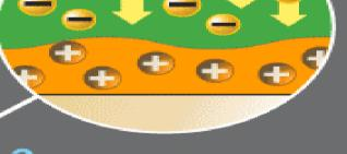
The holes jump to the emissive layer and recombine with the electrons. As the electrons drop into the holes, they release their extra energy as light.
